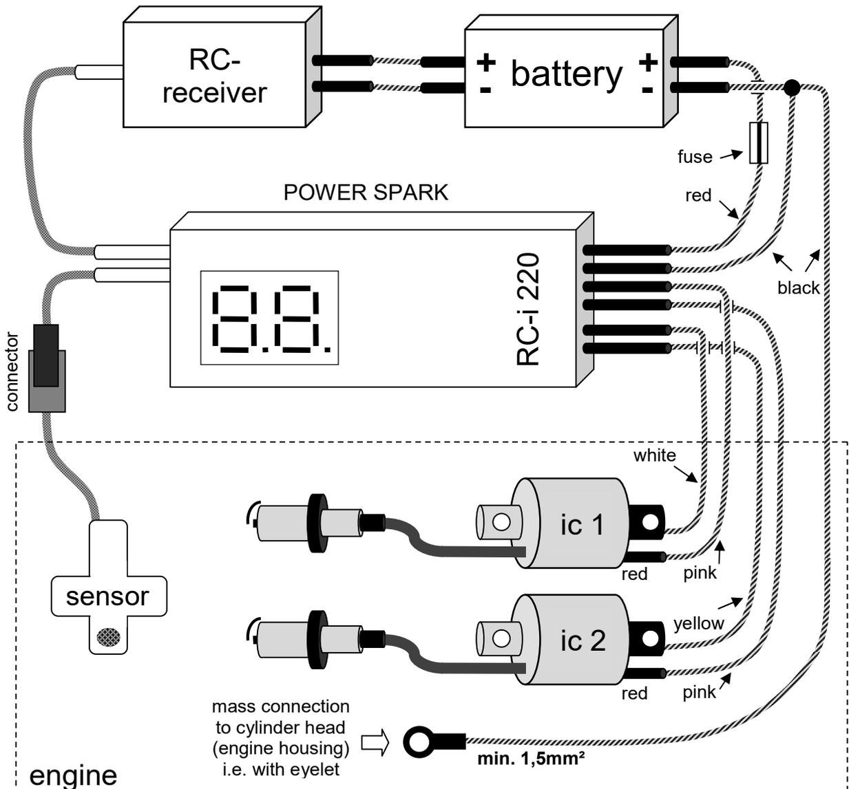
**important:** → make sure there is a low-resistance connection between battery minus and cylinder head (engine housing)
