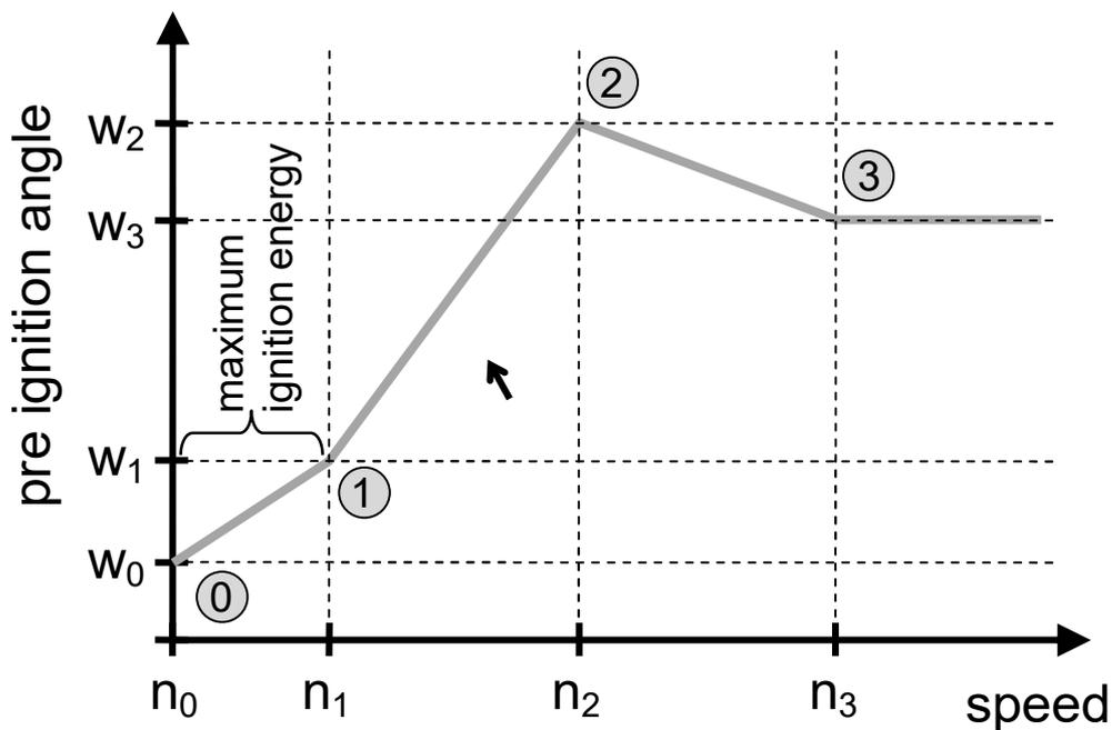
The speed values  $n_x$  can be adjusted in 100rpm- steps, the pre ignition angles in  $1^\circ$ -steps.
