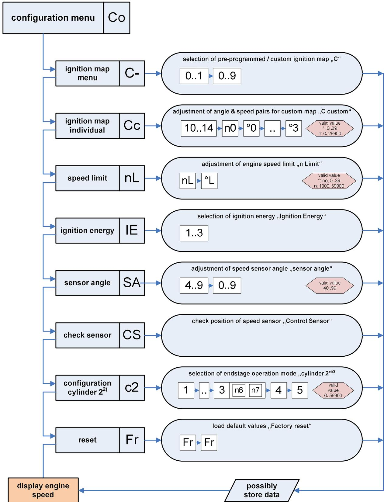
1) Only versions with diagnostic functions RC-i x2x, 2) only multiple cylinders versions RC-i 2xx & RC-i 4xx
