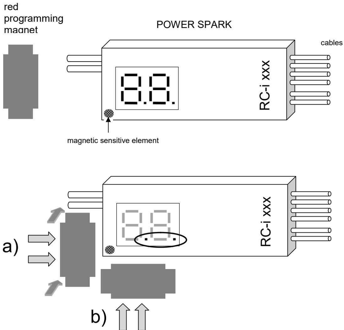
By approaching the programming magnet parallel to the **left side** of the POWER SPARK (sideways or from top, position a) ) in a distance of less than 10 mm the magnetic sensitive element is triggered. The POWER SPARK confirms the activation and shows „ . . “ additional to the active display.
