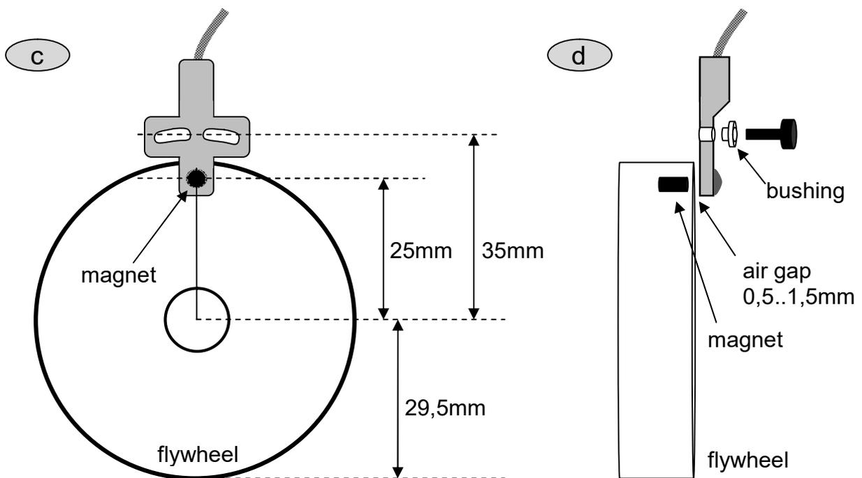
**→ HINT:** For fine adjustment use menu „control sensor” (p.38 & p.37) in the configuration menu.
