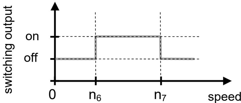
**Adjustment of speed threshold values**
