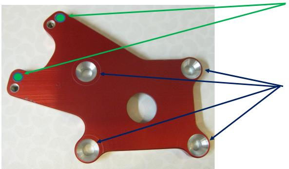
Later you have to use the green marked upper threaded bores for sensor holder fixation
